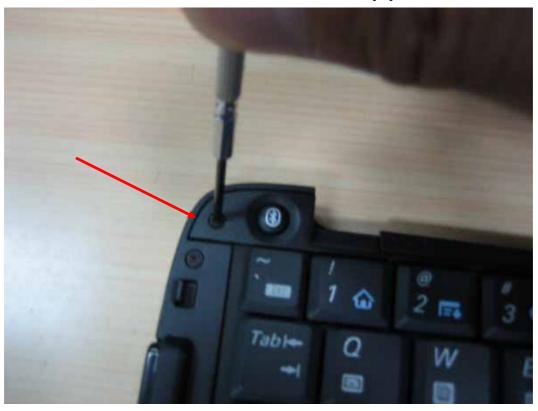
The left strip panel is disassembled
